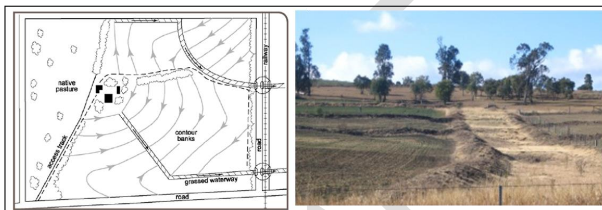
Figure 7: Left: Example of contour bank layout on a banana farm (Source: Figure 7.1, Chapter 7 Soil Conservation Guidelines). Right: Example of well-maintained contour banks on a Queensland farm (Source: https://www.qld.gov.au/environment/land/management/soil/erosion/management ).
